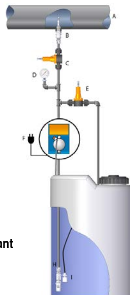
Fig.5 – Bleed operation for priming
